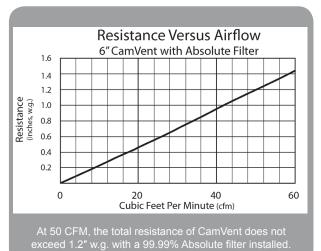
The Camfil CamContain CamVent is a slim and compact HEPA air filtration system.
